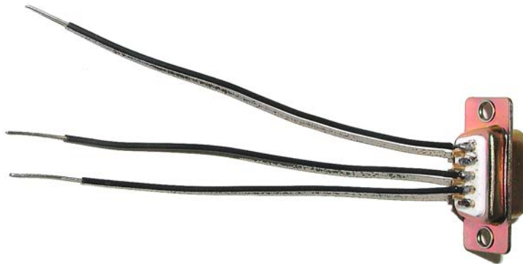
Solder Wires to back of male DB9 connectors
