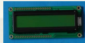
2. 1602 LCD (with backlight)
